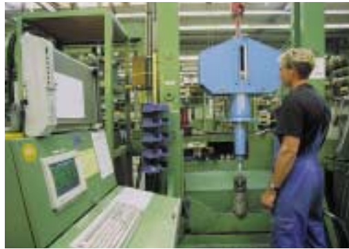
Acceptance test of a constant hanger
