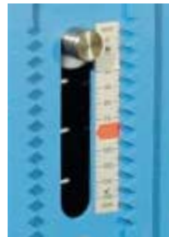
Travel scale with cold/hot markings
