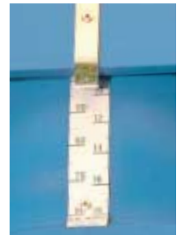
Load scale with indicator
