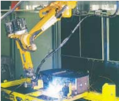
Modern welding robots and CNC machines ensure constant product quality
